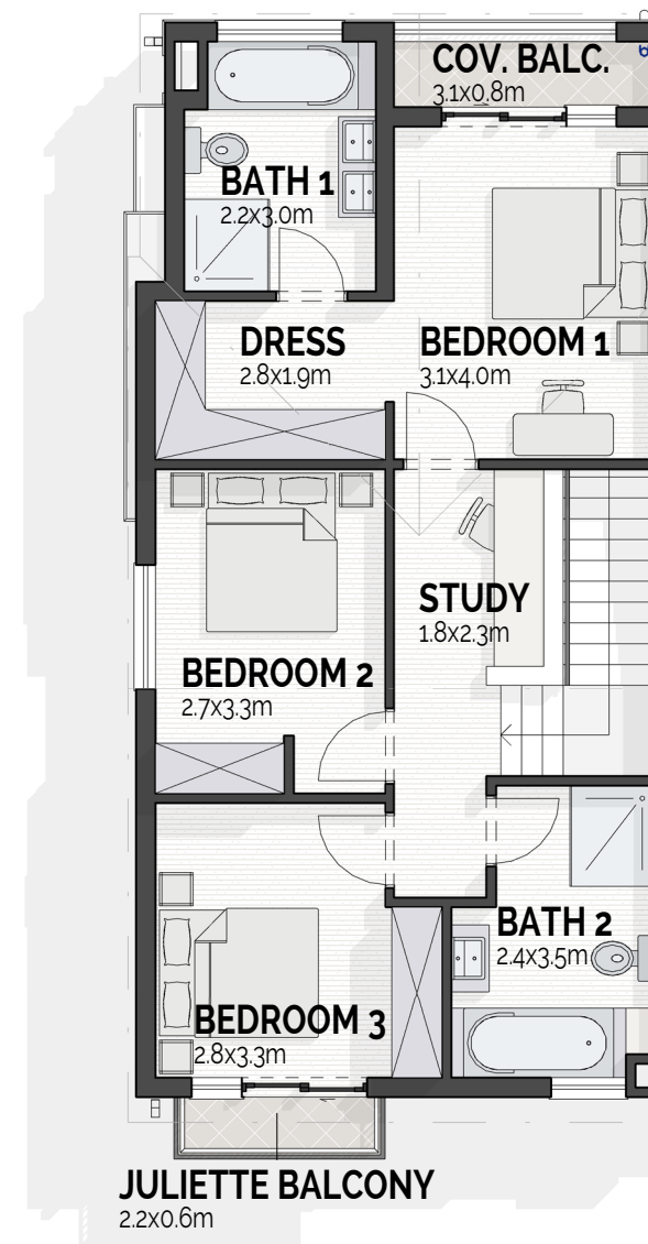
FIRST STOREY PLAN SCALE 1:100 ON A3 PAGE NORTH ORIENTATION AS PER SITE PLAN
