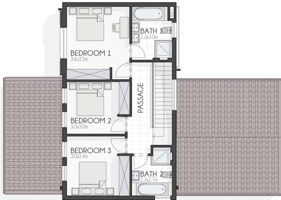
FIRST STOREY PLAN SCALE 1 : 100 ON A3 PAGE NORTH ORIENTATION AS PER SITE PLAN
